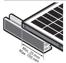
Rail length under module 25 - 100 mm
